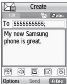
1. To change the text input mode, press the **Right** soft key.
