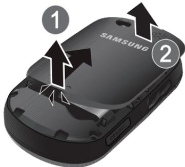
2. Carefully lift the battery cover away from the bottom of the phone.
