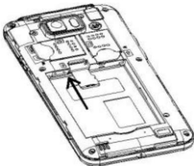
3. Finally insert the battery and the rear cover of the mobile phone.
