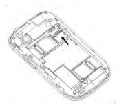
Insert the battery by aligning the gold contacts on the battery with the gold contacts in the battery compartment. Gently push down on the battery until it clicks into place.
